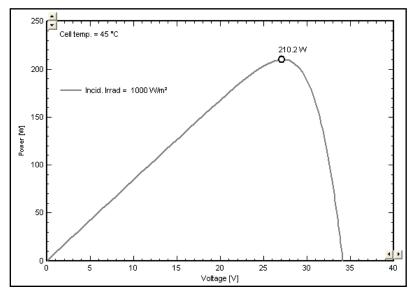
Power vs Voltage with main parameter of module temperature (T= 40 - 45 degrees Celsius)
